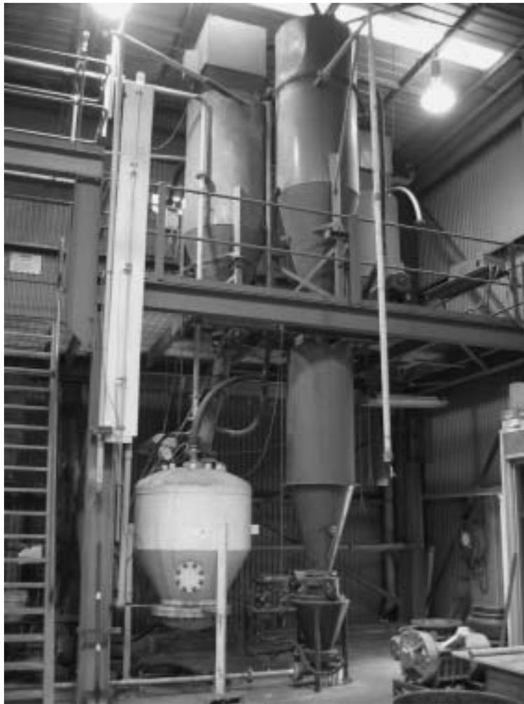
**Figure 5.13** Pilot test plant using a blow tank as a feeder.
