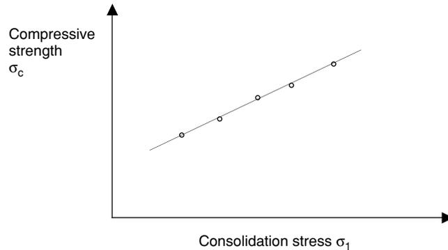
**Figure 2.8** Compressive strength vs. consolidation stress.
