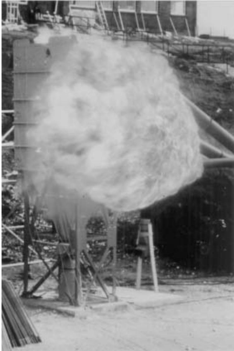
**Figure 6.1** Vented explosion in a dust collector. Reproduced with the permission of DCE Donaldson Ltd.
