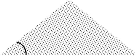
**Figure 2.1** Poured angle of repose.
