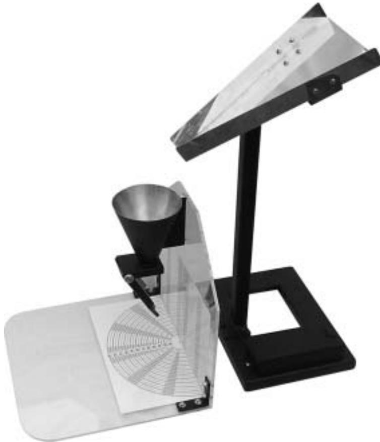
**Figure 4.1** Equipment for measuring the angle of repose,  $\alpha$ .
