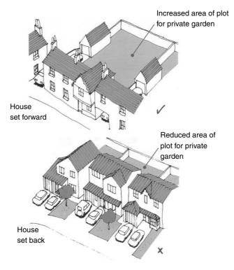
**Figure 3.1** Essex design guide (EPOA, 1997) – recommended dwelling arrangement for layouts at densities over 20 dph. Source: Essex County Council.
