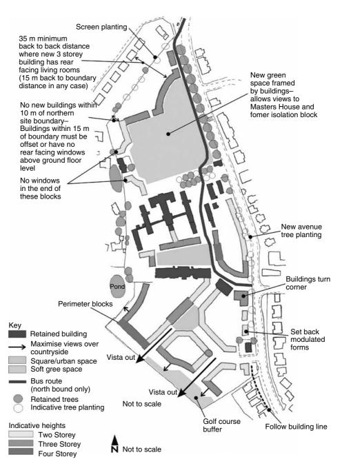
**Figure 3.11** St John's Hospital brief (CBC, 2006) – indicative layout. See also Plate 3.6. Reproduced with the permission of Chelmsford Borough Council and the Ordnance Survey on behalf of HMSO. © Crown copyright 2007. All rights reserved. Licence number 100046642.
