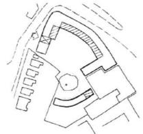
3. Potential for ground floor car parking beneath buildings. *Nb. Depth of Parkway* building allows active frontage to be incorporated in front elevation
