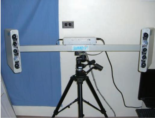
**Figure 4.3** The 3dMD stereo photogrammetric scanner (3dMD, Atlanta, Georgia). It consists of an array of digital cameras used to perform surface imaging of the patient’s face. A quick scan will generate a clinically accurate three-dimensional digital model of the patient’s face.
